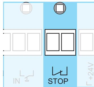
The status LED for STOP lights up green when the contact is closed.
