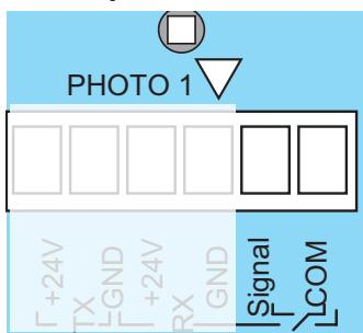
Connect the 2-wire photocell to the terminal block (PHOTO 1). The polarity is optional.
