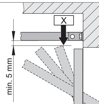
Fig. 1.1 Highest running point for one piece and up-and-over doors
