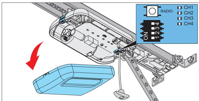
2. Remove the cover of the motor carriage.
