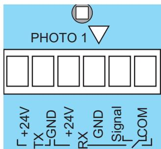
Connect the 4-wire photocell to the terminal block for door CLOSE (PHOTO 1). The supply for RX (Receiver) should be on the side facing away from the sun.
