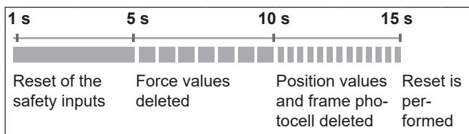
Fig. Overview of the time sequence of the ceiling control unit status LED when pressing the green Reset button
