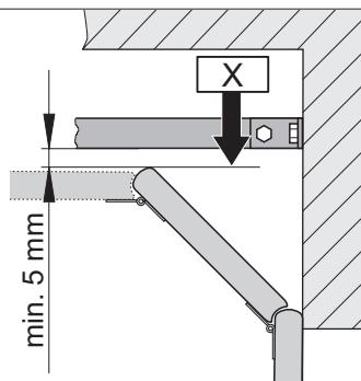
Fig. 1.2 Highest running point for a sectional door
