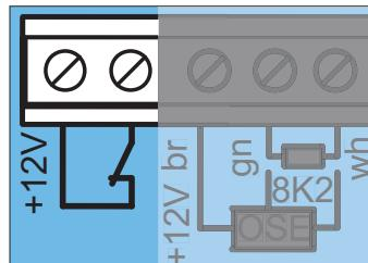
The wicket door safety device prevents operation of the door with an open wicket door. The wicket door safety device from **SOMMER** meets the requirements of EN 12453.
