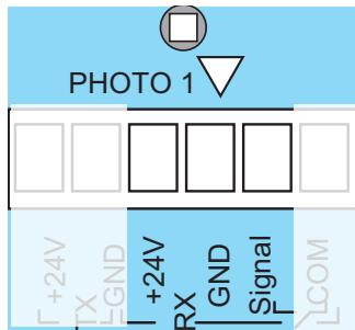
Connect the light curtain for door CLOSE to the terminal block (PHOTO 1).
