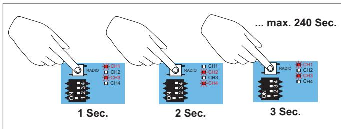
4. Count off the hold open time by counting the alternations of the LEDs. Release the Radio button when the desired duration has been reached.
