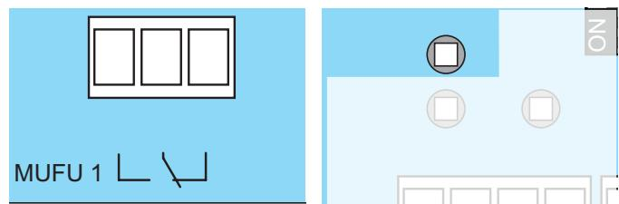
The status LED for MUFU 1 lights up green when the relay is energised.
