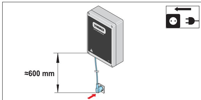
In order to connect to a power outlet or to an all-pole mains circuit breaker, e.g. a main switch, the wall control unit **must** be installed as follows:
