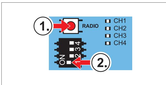
3. First, **press and hold** the Radio button. With the button pressed, set DIP switch 1 to "ON" position.
