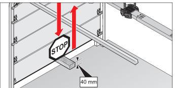
Fig. Example: Obstacle detection on sectional door
