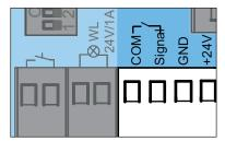
Fig. Terminal block for a 4-wire photocell
