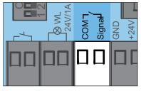
Fig. Terminal block for a 2-wire photocell
