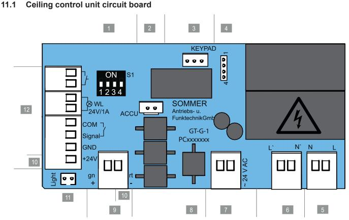
Fig. Ceiling control unit circuit board, complete version\*
