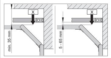
Fig. 1.2 Highest running point for a sectional door
