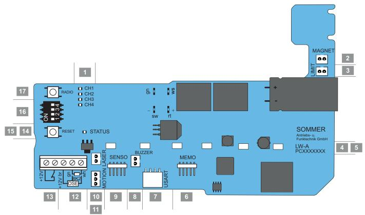
Fig. Motor carriage circuit board, complete version\*
