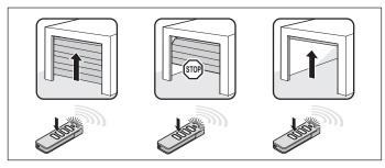
Fig. Pulse sequence for defined door OPEN
