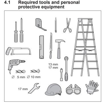
Fig. Recommended tools and personal protective equipment for installation
