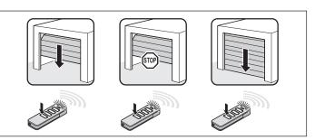
Fig. Pulse sequence for defined door CLOSE
