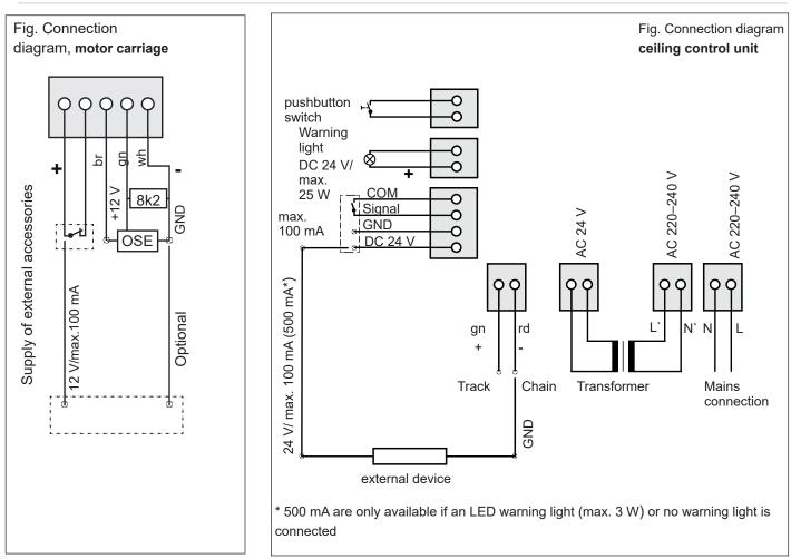
• When connecting external devices, power-saving mode must be deactivated to ensure the power supply.
